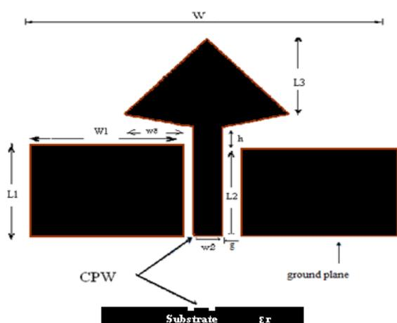
**Figure 20: The Layout of Ultra Wideband Coplanar Waveguide-fed Cedar Patch antenna.**
