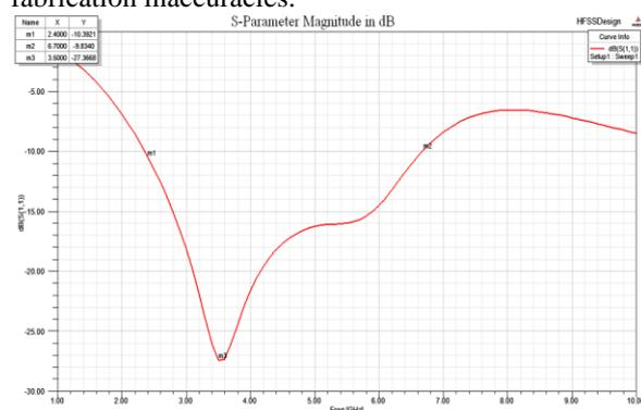
Figure 15: Simulated Return loss plot for Diamond shaped Compact antenna.
