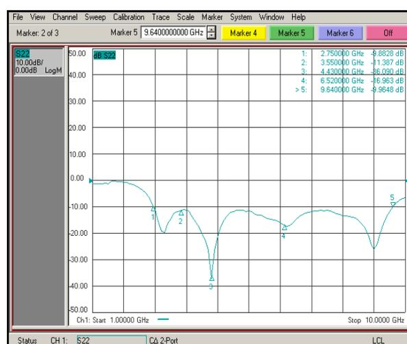
Figure 29: VNA Return Loss plot of Rectangular slot antenna with U-shaped tuning stub.
