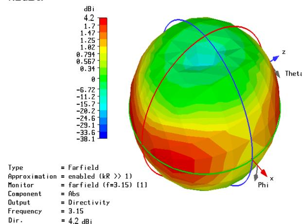
Figure 25: Bidirectional Radiation Pattern.
