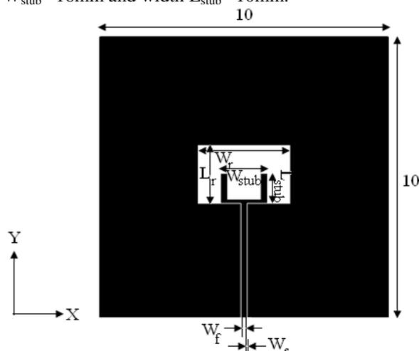
Figure 27: Layout of Ultra Wideband Coplanar Waveguide-fed Rectangular slot antenna. (All dimensions in mm)
