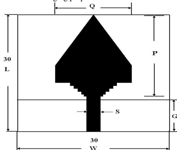
Figure 14: Top-View of the Diamond shaped Compact antenna (all dimensions are in mm).
