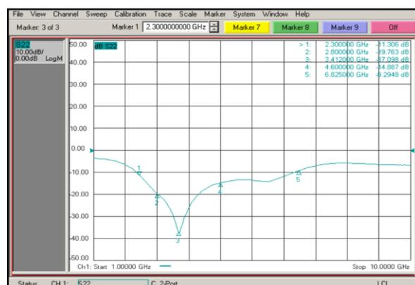
Figure 16: Measured VNA Return loss plot of Diamond shaped Compact antenna.
