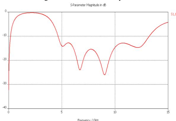
Figure 23: Simulated Return loss plot of UWB Cedar patch antenna.
