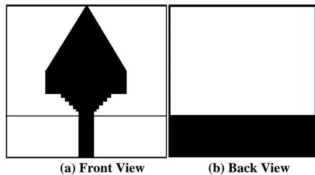
Figure 13: The Diamond shaped Compact antenna (Photo Plot).
