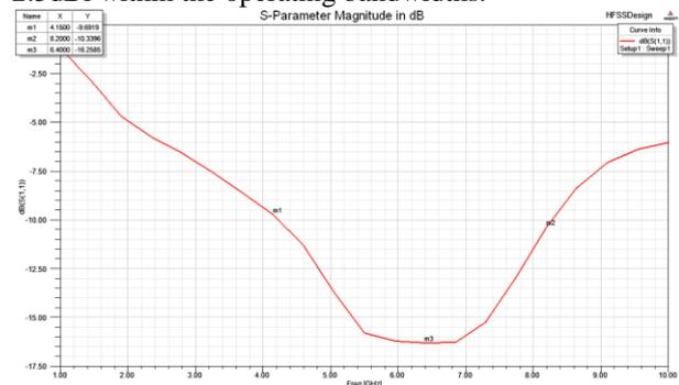
Figure 9: Simulated Return loss plot for Triangle patch antenna with Triangular slot.
