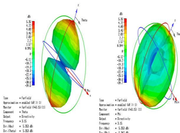
Figure 30: Three-dimensional Radiation Pattern, Theta cut and the Phi cut.
