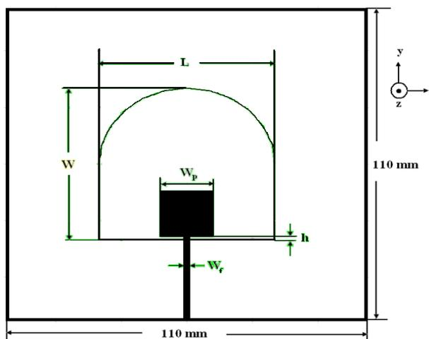
Figure 3: Top-View of the Square patch antenna with Wide slot (Design 1).
