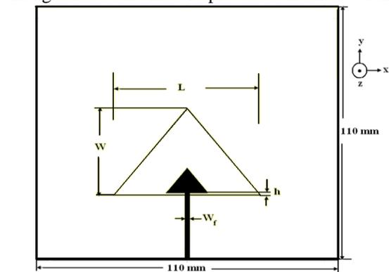
Figure 8: Top-View of the Triangle patch antenna with Triangular slot (Design 2).
