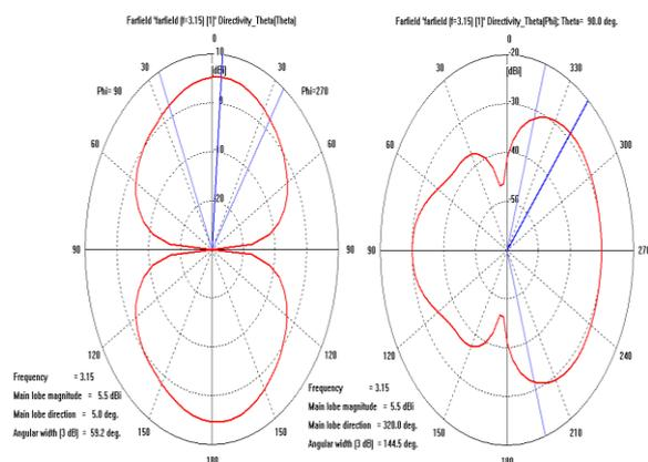
Figure 31: Polar Radiation Pattern, Theta cut and the Phi cut.
