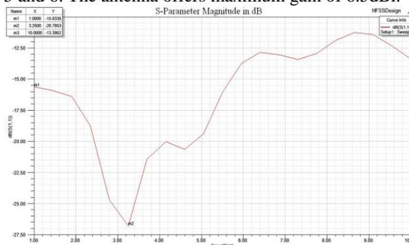
Figure 4: Simulated Return loss plot for Square patch antenna with Wide slot.
