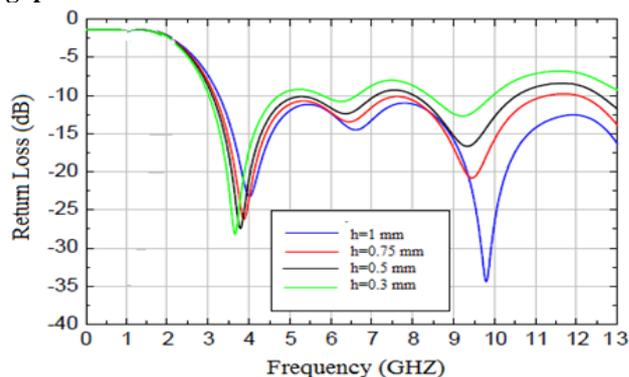
**Figure 21: Return loss v/s frequency as a function of 'h'.**
