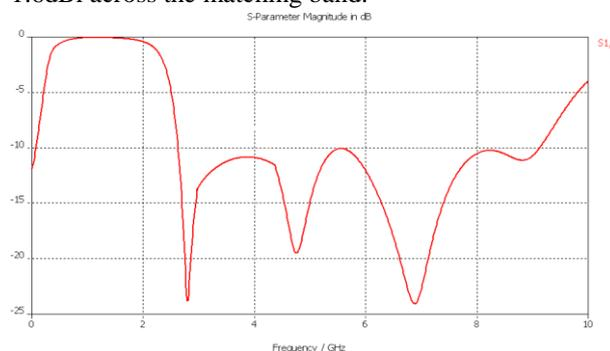
Figure 28: Simulated Return loss plot of Rectangular slot antenna with U-shaped tuning stub.
