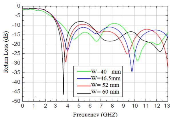
Figure 22: Return loss v/s frequency as a function of 'w'
