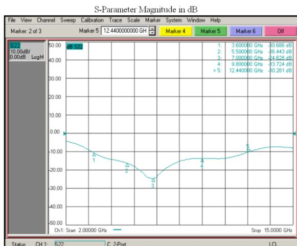
Figure 24: VNA Return Loss plot of UWB Cedar patch antenna.
